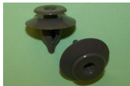
78020P QTY20 Trim fastener for .090" board thickness and snap-fit in 21/64" diameter panel hole. All early Fords. N.B. FIX37 is same dimensions but in white
