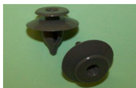
78020P QTY:20 Trim fastener for .090" board thickness and snap-fit in 21/64" diameter panel hole. All early Fords. N.B. FIX37 is same dimensions but in white
