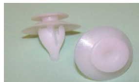
FIX37P QTY:20 Panel Clip, White. 18mm diameter to fit 8mm hole. Suits Ford and VW N.B. 78020 is same dimensions but in grey
