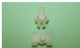
BSF282P QTY:15 Side moulding clip for a 11.5mm moulding gap and a 7.0mm panel hole. Mercedes and general application. Mercedes part no. 0009902192
