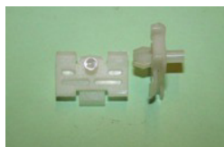
BSF282P QTY:15 Side moulding clip for a 11.5mm moulding gap and a 7.0mm panel hole. Mercedes and general application. Mercedes part no. 0009902192
