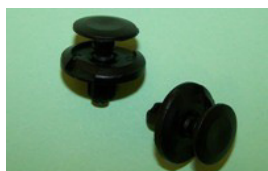
AP4683P QTY:12 Wing Mudguard Push-Type Retainer, (head dia : 20mm, stem : 10mm, to fit hole:7mm) Black. Fiat / Suzuki / Toyota: Camry, Echo, MR2 & Sienna 1997 – ON Fiat part no. 71741883
