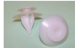
FIX37P QTY:20 Panel Clip, White. 18mm diameter to fit 8mm hole. Suits Ford and VW N.B. 78020 is same dimensions but in grey
