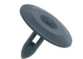
FIX59P QTY:23 Trim Button head size 25.0mm and panel hole 6.0mm in black. Audi and general application
