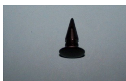
WBU060 QTY:20 Arrow clip, head size 12.5mm, material thickness 0.8mm-6.8mm, panel hole 6.55mm, plain head. Rover and general application.
