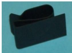
27760P QTY:10 'S' type edge clip for 2.4mm and 5.5mm material thicknesses. Depth 17mm and Width 12.7mm. Not barbed. Triumph Stag seat back.
