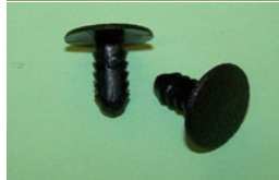
FIX30P QTY: 25 Trim Button, head size 17.0mm, material thickness 1.0mm-15.0mm and panel hole 6.0mm. Multi-step, black. General Application
