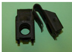
BSF272P QTY:6 'J' Nut retainer for M12 Screw, standard reach. Panel thickness 5.6 - 6.3mm. General application.
