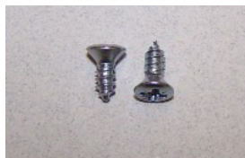
BSF181P QTY:35 No.6 x 1/2" domed, countersunk, posidriv, self tapping screw in steel General application.
