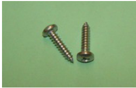
BSF148P QTY:20 No.8 x 3/4" pan-headed, posidriv screw in stainless steel. General application.
