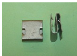
38201P QTY:25 'S' type edge clip for 0.2 - 1.2mm and 1.8 - 2.1mm material thicknesses. Depth 11.9mm and width 12.7mm. General application.
