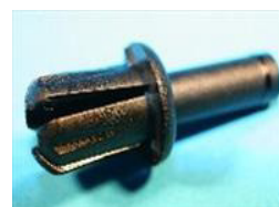
BSF092P QTY:26 Plastic expansion rivet panel thickness 0.8 - 9.5mm. Hole diameter 8.0 - 8.5mm. General application
