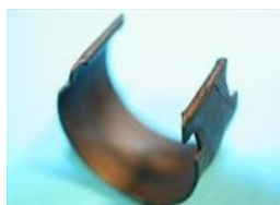
13780P QTY:22 Trim retaining clip for 13/16" diameter tubular seat frames. Jaguar, Triumph, Ford, Hillman and general application.
