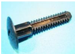
77561P QTY:10 Ratchet Type quick release fastener, panel thickness 8.2mm-30.3mm, panel hole 8.5mm. General application.
