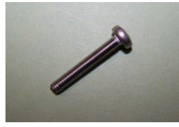
BSF145P QTY:20 M4 x 20mm pan-headed, posidriv screw in stainless steel. General application.
