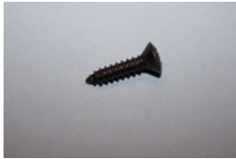
BSF038P QTY: 35 No.8 x 3/8" self-tapping screw. Domed posidriv, countersunk head in black. General application
