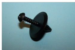
SCR033P QTY:12 Screw rivet, open end type. 5.0mm material thickness, head size 26.3mm and 6.3mm panel hole. Ford Cortina, Granada, Capri, Escort insulation clip.
