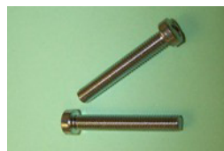
BSF247P QTY:12 1 1/4" x 2BA pozidriv with a Filister head in Chrome. Morris 1000 inner door handle and general application
