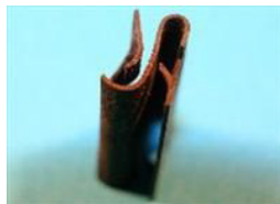
22970P QTY:20 'S' type edge panel removeable clip, height 8.0mm, panel thickness 1.2mm and 1.6mm. General application.
