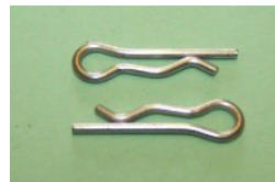
BSF199P QTY:25 Brake Hardware- 'R' clip 1.5mm dia wire, for front caliper kits. Ford, Vauxhall and general application.
