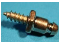
952P QTY:6 Lift the Dot stud with 3/8" x No. 10 self tapping screw used with Part Nos. 608 and 708A combination. General application.
