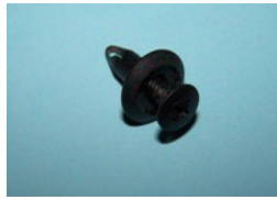
BSF144P QTY:12 Screw rivet, closed end type, 2.5mm-8.0mm material thickness, head size 15.5mm and 6.5mm panel hole. General application.
