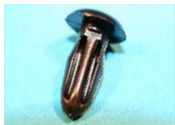
71650P QTY:30 Snap-in stud for 3/16" diameter panel hole and 3.2 - 4.8mm material thickness. Ford Cortina bonnet flip seal and general application
