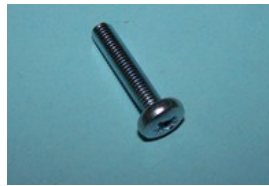
BSF097P QTY:15 M5 x 25mm pozidriv pan- headed in steel. General application.
