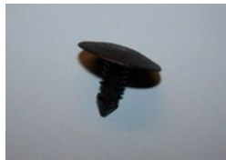
FTB011P QTY:25 Fir Tree Button for 7.2mm diameter panel hole and material thickness 2.5-9.0mm. Head diameter 24.00mm. Colour black with a grained head. General application.
