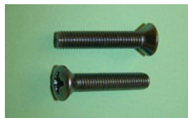
BSF252P QTY:12 1/4" UNF x 1 1/4" screw: raised, countersunk, pozidriv head in mild steel. General application.
