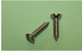
BSF019P QTY:20 No. 8 x 3/4" domed, countersunk, slotted, self-tapping screw in stainless steel. Mini headlamp surround and general application.
