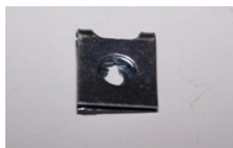
SNU1686P QTY:30 'U' nut for No.8 self-tapping screw. Length 14.0mm, width 12.7mm. General application.
