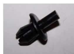
DRR057P QTY 25 Plastic expansion rivet, panel thickness 4.0-7.0mm. Hole diameter 7.9-8.5mm. Head diameter 16.0mm. Vauxhall range and General application.
