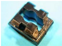
73220P QTY:19 Quarter Turn Cam, panel thickness 1.2mm. Mini, Triumph and general application.
