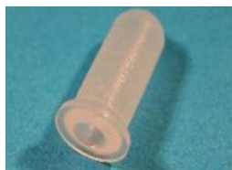
80670P QTY:45 Plastic fix for 1/8" diameter pin in 3/16" panel hole. General application
