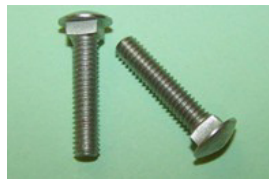
BSF279P QTY:8 8/32 UNC x 1" Flat head, squared screw. Early Ford rear light assemblies and general application.
