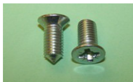
BSF246P QTY:15 1/4" BSF x 5/8" Countersunk, posidriv, with a point, in zinc plated steel. Morris 1000 lock assembly and general application
