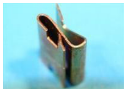
11516P QTY:32 'S' type edge clip for 0.75 - 1.25mm and 2.0 - 2.3mm material thickness. General application.
