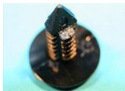
FTB017P QTY:30 Grained headed fir tree clip for 6.0mm panel hole and material thickness from 3.0mm - 8.0mm. General application.
