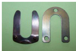
BSF198P QTY: 4 Brake Hardware- Bowed Horseshoe Clips for rear wheel cylinder (pack includes 2 pairs- sufficient for one car). Girling Type 75. Early Fords, Triumph.
