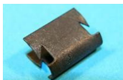
11950P QTY:35 Edge clip 8.7 height, for material thickness of 3.2- 3.6mm, width 12.7mm. General application.
