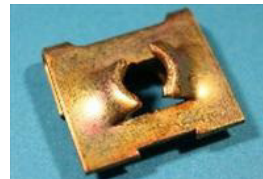
SNJ1861P QTY:30 No14 'J' nut, length 17.8mm, width 19.3mm (short reach). General application Austin-Morris part no. 518454 Standard-Triumph part no. FA3057/4
