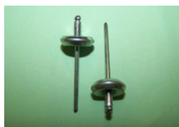
BSF077P QTY:10 Round 'Tuckers' moulding clip for 14mm moulding gap and 3.2mm panel hole. Early Fords, Triumph, Sunbeam Alpine and general application.
