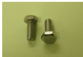
BSF238P QTY:20 1/4" BSF x 5/8" HT Hex Set Screw in zinc plated steel. Morris 1000 and general application
