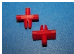
12724P QTY:30 Moulding clip for 8.0mm moulding gap and 6.5mm panel hole. VW Golt Mk1 Sill and general application.
