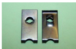
SNU1561P QTY:25 'U' nut for No.8 self-tapping screw. Length 24.4mm, width 11.2mm, standard reach. General application.
