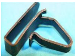
14480P QTY:30 Door trim pad clip for .100" board and snap fit in 1/4" panel hole. Triumph Herald, Spitfire, TR6,GT6, Jaguar, Minor 1000 & general application.
