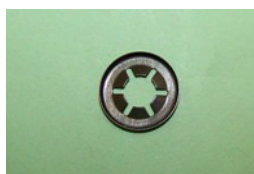
PUN007P QTY:25 Circular push on ratchet plate 5mm stud diameter. Outside Diameter 11.3mm. General application.
