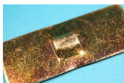
BSF059P QTY:12 Backplate for 2-piece moulding clip measuring 1.3/4" x 3/4". Used with Part No. 11480 spring retainer and intended for do-it-yourself modification to suit the moulding profile. General application.
