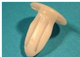
71790P QTY:25 'W' button for material thickness 3.2 - 4.8mm and panel hole 7.1mm. General application.
