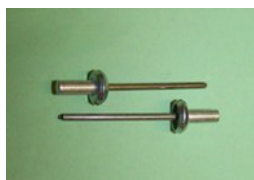
BSF079P QTY:18 Round 'Tuckers' moulding clip for 7.0mm moulding gap and 3.2mm panel hole. Jaguar, Vauxhall, also Triumph Stag Hardtop (front) in metal (for plastic see 72650.),
