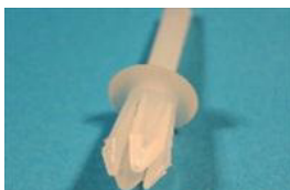
.80830P QTY:20 Expansion rivet panel thickness 2.4mm - 7.8mm. Hole diameter 5.5mm - 6.5mm. General application.
