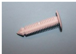
BSF105P QTY:25 Fir Tree Button for 7.2mm diameter panel hole and material thickness 2.3-30.00mm. Head diameter 16.4mm. Colour White. General application.
