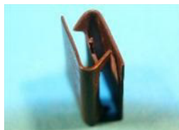
19190P QTY:26 'S' type edge clip for material thicknesses 1.0mm - 2.0mm and 1.4mm - 2.00, and 8.7mm depth. General application.
