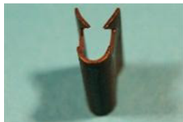
11560P QTY:35 Edge clip 8.7mm height ,for material thickness of 2.0- 2.8mm, width 12.7mm. General application
