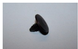
FTB064P QTY:20 Fir Tree Button for 5.0mm diameter panel hole and material thickness 1.2-6mm. Head diameter 16.0mm. Colour black with a matt head. General application.
