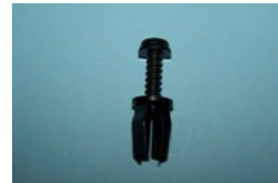
SCR017P QTY:15 Screw rivet, open end type. 4.0mm material thickness, head size 12.0mm and 9.0mm square panel hole. Ford Escort, Fiesta tailgate.
