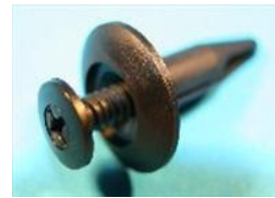
BSF109P QTY:10 Screw rivet, closed end type, 2.5mm-8.0mm material thickness and 6.5mm panel hole. General application.
