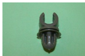
CAC240P QTY:15 For 5/16" diameter pipe in grey. Ford.
