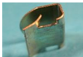
16460P QTY:30 'D' type edge clip height 9.0mm, for material thickness of 2.8mm. General application.
