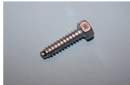
BSF023P QTY:15 6.3mm x 25mm type 'E' blunt point screw with hexagon head in steel. Used with SNJ1761 and SNJ1861 and general application.
