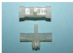
12869P QTY:24 Moulding clip for 5.5mm moulding gap and 4.4mm panel hole. Mini Estate.
