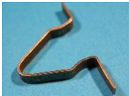
11480P QTY:23 Spring retainer for snap fit in 7.2mm panel hole and for total material thickness of 4.0mm. Minor 1000 and general application..
