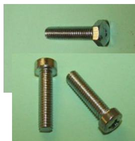
BSF248P QTY:15 3/4" x 2BA pozidriv with a Filister head in Chrome. Morris 1000 window winder handle and general application
