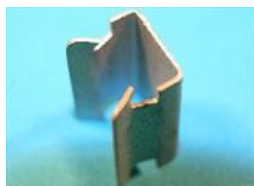
BSF091P QTY:15 Edge panel clip, height 9.5mm for 9.0mm-9.5mm material thickness. General application.
