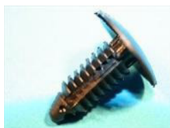
FTB055P QTY:30 Fir Tree Button, material thickness 2.3 - 14.2mm, head diameter 17.8mm, panel hole 6.4mm. General application. Colour black.
