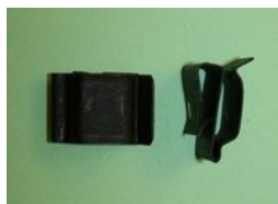
CAC253P QTY:20 Edge cable/pipe clip for twin 3/16" diameters and 0.6-4.5mm panel thickness. Ford Capri MK1 and general application.
