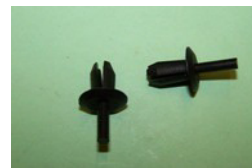
BSF215P QTY:30 Drive rivet, 12.5 head size, length 10mm and panel hole 6mm. Ford Granada 85-98 Windscreen scuttle ( see BSF214P below) and general application.
