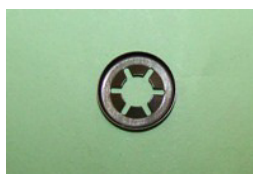
PUN009P QTY:25 Circular push on ratchet plate 5mm stud diameter. General application. Outside Diameter 15mm.
