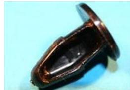
WBU016P QTY:35 'W' Button, head size 14.0mm, material thickness 0.8mm-5.9mm, panel hole 7.0mm, plain head. General application.
