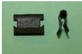
.13710P QTY:55 Edge clip 8.7mm height ,for material thickness of 0.8 - 2.0mm, width 12.7mm. General application.
