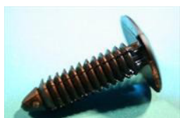
FTB056P QTY:27 Fir Tree button for 1/4" diameter panel hole and for material thicknesses from 2.8 - 20.3mm. Colour black (was PC47564) General application.
