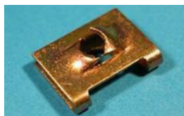
SNU3275P QTY:30 'U' nut for No.10 self tapping screw - short reach. General application.
