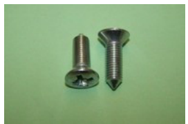
BSF206P QTY:8 5/16" UNF x 1" screw: raised, countersunk, pozidriv head in mild steel. General application
