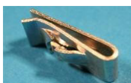
SNU3381P QTY:25 No8 'U' nut, length 16.5mm, width 8.6mm. General application and Ford Escort.
