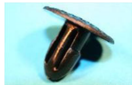
75810P QTY:24 Snap-in stud for 1/4" diameter panel hole and 3.7mm material thickness. General application.
