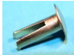
BSF095P QTY:25 Bifucated rivet 5/16" (8.0mm) head size, 3.8mm diameter and 11.0mm in length. General application.
