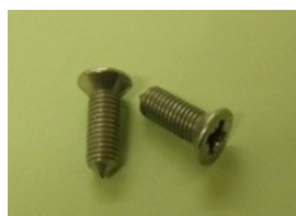
BSF240P QTY:10 5/16" BSF x 15/16" Countersunk, posidriv, with a point, in zinc plated steel. Morris 1000 and general application
