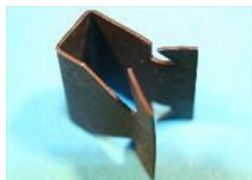
18670P QTY:30 Edge clip for material thickness 3.2mm - 5.1mm and 12.7mm depth. Jaguar XJ6
