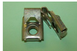
BSF086P QTY:10 'J' Type retainer for a 5/16" UNF thread, standard reach. General application Standard-Triumph part no. FQ3404/4
