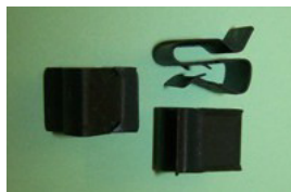
BSF250P QTY:20 Edge cable/pipe clip for twin 3/16" diameters and 2.0-4.7mm panel thickness. General application. Standard-Triumph part no. 618386.
