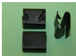
33100P QTY:30 'S' type edge clip for 2.2mm and 2.9mm material thicknesses. Depth 9.7mm and width 12.7mm. General application.
