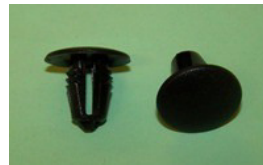
FIX35P QTY:25 Trim Button, head size 18.0mm and panel hole 8.0mm in black. Ford under-dash felt, and General application
