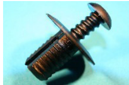
BSF108P QTY:10 Screw rivet, open end type, 3.0mm-10.0mm material thickness and 8.0mm panel hole. General application.
